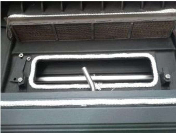
6. Run a small bead of gasket glue ( about  $\frac{1}{8}$ " inch) all around the gasket channel. Again, starting in the middle of the front, lay the gasket in the channel, being sure to fill the corners completely. Tuck the two ends together. Use the putty knife to tuck in any loose ends.
