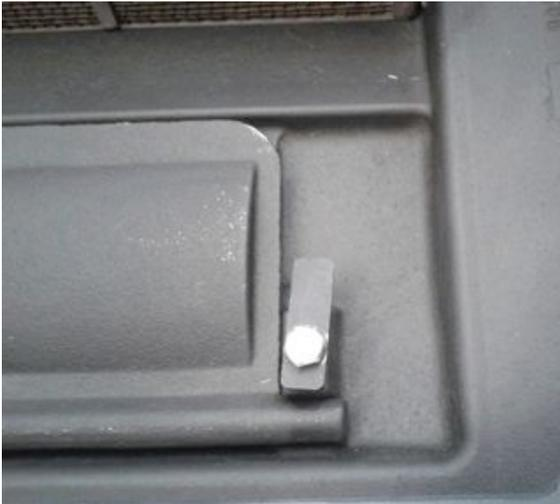
Bypass retainer nut is loosened so it can 'swing' out of the way for removal of bypass door.
