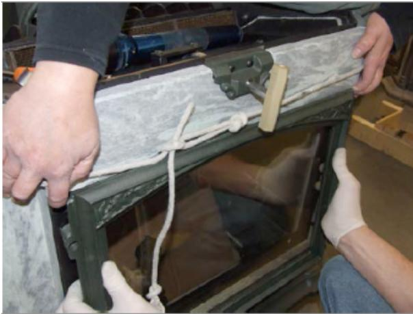
6. Note: The assembly consists of a cast iron frame and two panes of glass. On top of the assembly sits the ‘over the front stone’ that will also come loose when the front assembly is removed. If the stone is dropped it may result in damage. One person should hold the stone upward while the other removes the front assembly. The stone can then be set aside.
