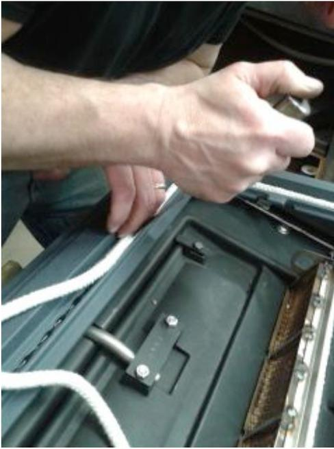
6. When you get to the starting point, back up the gasket just slightly to meet the beginning and tuck the ends in with the putty knife.
