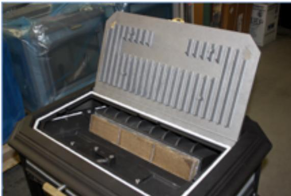
Take the top stones off the lid and lift the cast iron griddle top. Remove catalytic combustor to expose gasket area behind it.
