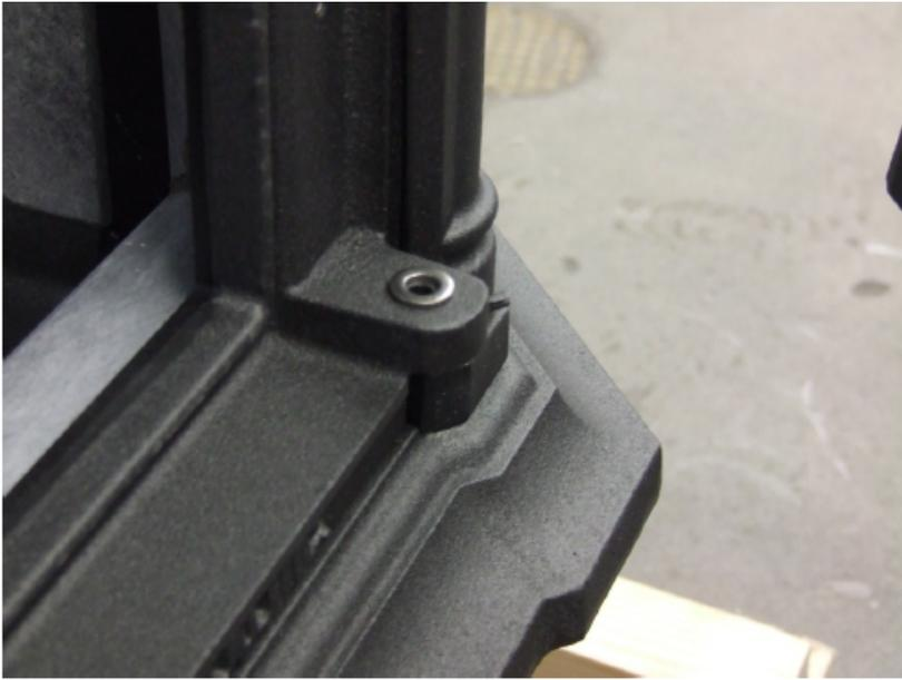
Note- there may be one or two small washers on the door-frame side of the hinge. These must be returned to their original location for proper alignment when the door is reinstalled (see photo)
