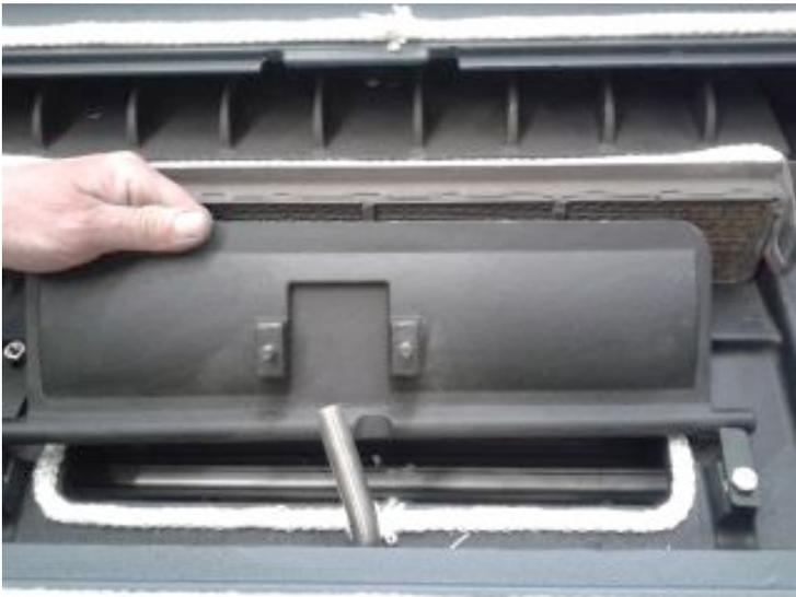
5. Remove the old gasket material and clean the channel. Dry fit the new gasket in the channel, starting in the middle at the front of the stove, under the bypass rod, making sure to completely fill the corners, continue around to meet the first end. Cut gasket about  $\frac{1}{4}$ " longer. Remove gasket and set aside.
